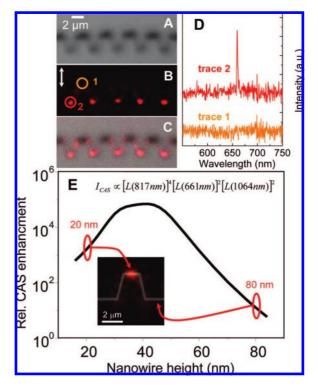
**Figure 4.** (A) Transmission image, (B) coherent anti-Stokes image, and (C) overlay image of nanozigzags. Emission spectra from the points 1 and 2 indicated in B are shown in D. Trace 2 is offset for clarity. (E) Calculated CAS enhancement as a function of nanowire height using the lightning rod model. Marked regions indicate the relevant heights of the nanozigzag structure. The local field enhancement factor L is calculated as in ref 21.
