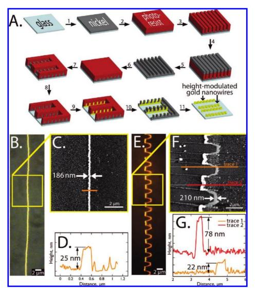
**Figure 1.** Fabrication and characterization of gold nanowires type I and type II. (A) Schematic of the fabrication method of height modulated nanowires (type II). (B) Dark-field transmission image of wire type I. (C) AFM image of wire type I, and cross-sectional profile (D) as measured with AFM. (E) Dark-field transmission image of wire type II, along with AFM image (F) and AFM cross-sectional profile (G).
