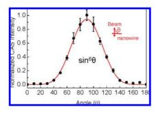
**Figure 3.** Polarization dependence of coherent anti-Stokes emission as a function of the angle  $\theta$  between beam polarization and longitudinal axis of the wire. The fitted line follows a sin<sup>6</sup>  $\theta$  angular dependence. Excitation and detection conditions are identical as in Figure 2.
