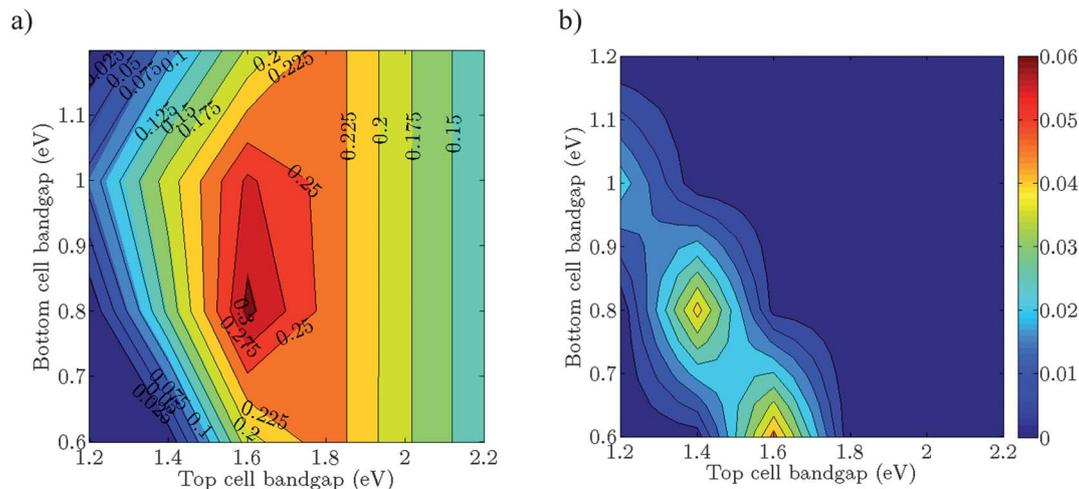
**Fig. 5** (a)  $\eta_{@I=1 \text{ kW m}^{-2}}$  (black lines) and  $\bar{\eta}_a$  (color lines), and (b)  $\sigma_a$ , as a function of the band gap of the bottom and top cells of the dual-absorber tandem cell for  $T = 300 \text{ K}$  for  $l_{\text{el}} = t_{\text{e}} = 1 \text{ cm}$  and  $\eta_{\text{pc}} = 1$ .
