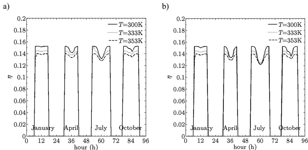
**Fig. 3** Efficiency of a PEC device for four typical seasonal days at three isothermal conditions ( $T = 300, 333, 353$  K), for the Si/GaAs dual-absorber tandem cells for Designs A and B with  $l_{el} = 50$  mm,  $t_e = 1$  mm, and  $\eta_{pc} = 1$ .
