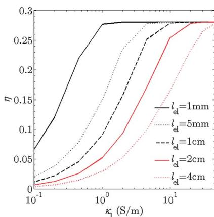
**Fig. 9**  $\eta_{@I=1 \text{ kW m}^{-2}}$  as a function of electrolyte conductivity for various electrode lengths,  $l_{el}$ , for  $t_e = 10 \text{ mm}$  and  $\eta_{pc} = 1$ , for top and bottom cell band gaps of 1.0 eV and 1.6 eV.
