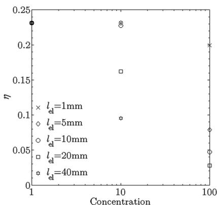
**Fig. 10**  $\eta_{@I=1 \text{ kW m}^{-2}}$  as a function of solar irradiation concentration for various electrode lengths,  $l_{el}$ , for  $t_e = 10 \text{ mm}$  and  $\eta_{pc} = 1$ , for top and bottom cell band gaps of 1.1 and 1.6 eV.
