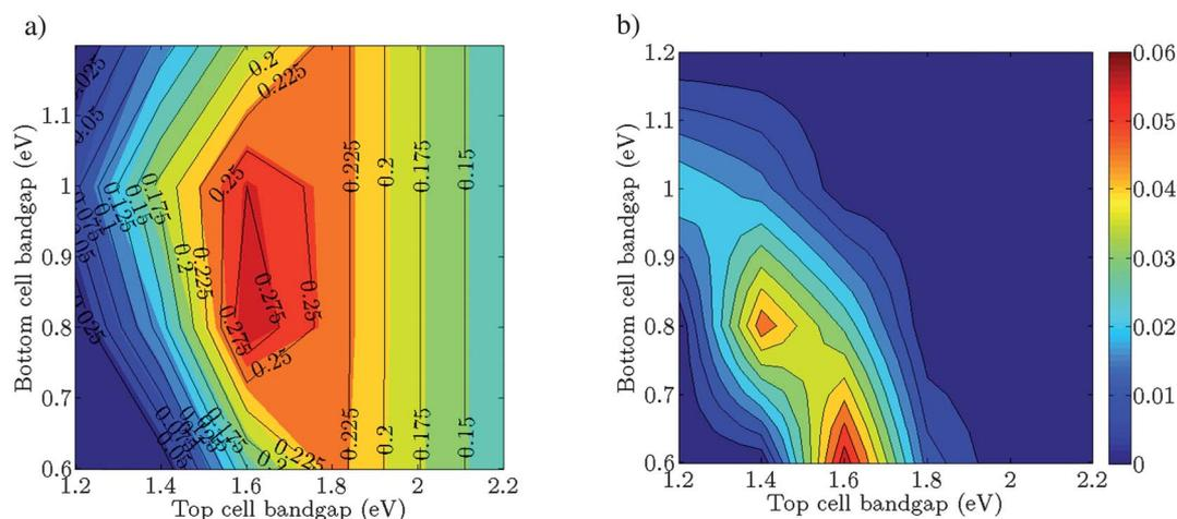
**Fig. 6** (a)  $\eta_{@I=1 \text{ kW m}^{-2}}$  (black lines) and  $\bar{\eta}_a$  (color lines), and (b)  $\sigma_a$ , as a function of the band gap of the bottom and top cells of the dual-absorber tandem cell for  $T = 353 \text{ K}$  for  $l_{\text{el}} = t_{\text{e}} = 1 \text{ cm}$  and  $\eta_{\text{pc}} = 1$ .
