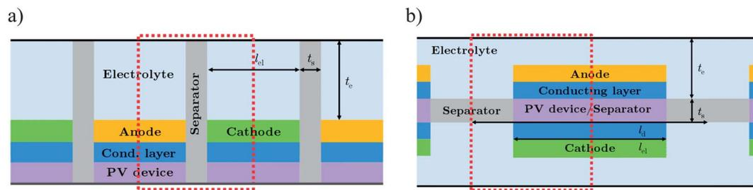
**Fig. 1** Schematic of (a) the side-by-side design (Design A), and (b) the top-to-bottom design (Design B) used as model devices, indicating the various dimensional variables, *i.e.* the electrode length, separator thickness, electrolyte height, and device length. The red dotted boxes indicate the modeled unit cells.
