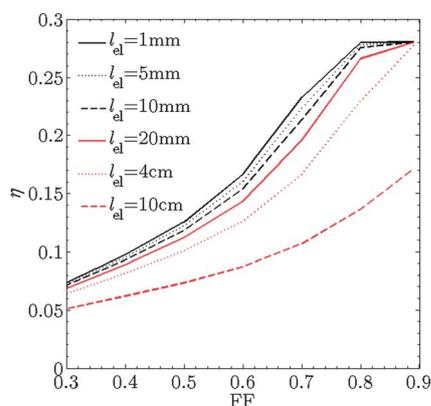
**Fig. 7**  $\eta_{@I=1 \text{ kW m}^{-2}}$  as a function of the fill factor of the dual-absorber tandem cell and the electrode length for Design B for  $t_e = 10 \text{ mm}$ , and 1.0 and 1.6 eV band-gap combinations for  $\eta_{\text{pc}} = 1$ .
