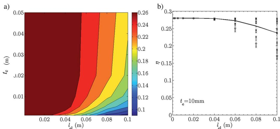
**Fig. 8** (a)  $\eta_{@I=1 \text{ kW m}^{-2}}$  as a function of electrode length,  $l_{\text{el}}$ , and electrolyte height,  $t_e$ , and (b)  $\eta$  (crosses) and  $\bar{\eta}_a$  (solid line) for  $t_e = 10 \text{ mm}$ . Both calculations used top and bottom cell band gaps of 1.0 and 1.6 eV for  $\eta_{\text{pc}} = 1$ . The circled crosses in (b) indicate  $\eta_{@I=1 \text{ kW m}^{-2}}$ .
