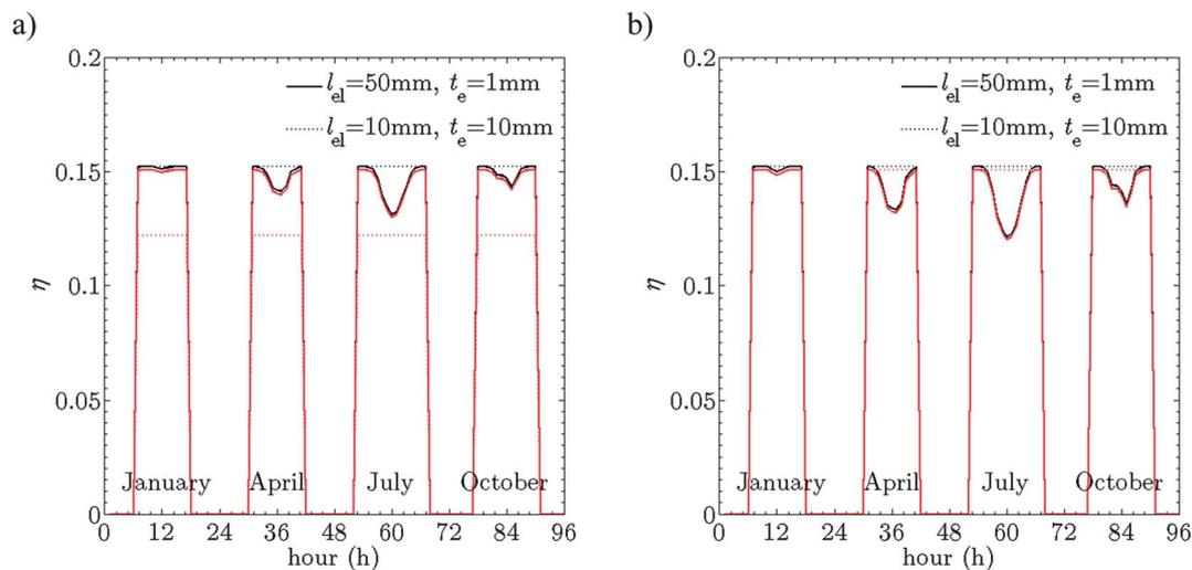
**Fig. 2** Efficiency variations of the device during four typical seasonal days for a realistic dual-absorber tandem cell, *i.e.* Si/GaAs multi-junction, for (a) Design A and (b) Design B for two combinations of device dimensions, with assumed  $\eta_{pc} = 1$  (black lines), and with  $\eta_{pc}$  calculated according to the species conservation equations (red lines).
