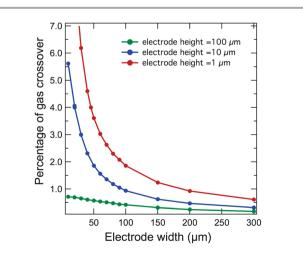
Fig. 7 Percentage of gas crossover as a function of the electrode width when the electrode height was set to 1  $\mu$ m (red), 10  $\mu$ m (blue) and 100  $\mu$ m (green).
