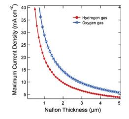
**Fig. 2** Maximum sustainable current density, as a function of the Nafion thickness, allowed to avoid supersaturation of oxygen (blue) or hydrogen (red) at the Nafion/catalyst interface in Design A.
