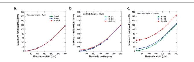
**Fig. 4** Maximum resistive loss as a function of the electrode width for three different electrode heights, 1 μm (a), 10 μm (b) and 100 μm (c), in Design A. Three fill fractions, 0.5 (green), 0.9 (blue) and 0.98 (red) were simulated for each electrode width.
