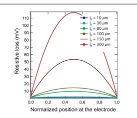
**Fig. 3** Resistive loss as a function of normalized position along the electrode for six different electrode widths in Design A.
